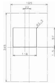
1mm clearance on each side of handle
