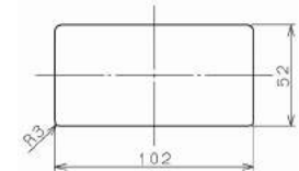
1mm clearance on each side of handle
